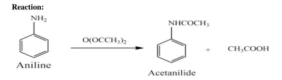
**Procedure:** Prepare mixture of aniline (12ml), acetic anhydride (12ml), glacial acetic acid (12ml) and zinc dust (0.1gm) is refluxed gently in a round bottom flask under anhydrous condition for 10-15 min. Pour the hot mixture with constant stirring to 200 ml of ice cold water in a beaker. Filter the product and wash with water, recrystallized from boiling water containing 3-4 ml alcohol. The yield is 12gm and M.P.is 114°C
